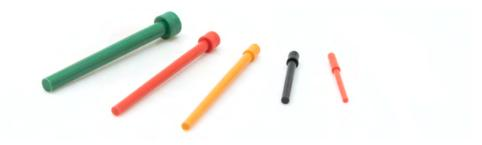
Sealing plugs are used to seal unwired contact cavities. After installing unwired contacts into unused cavities, insert knob end of sealing plug into grommet until it bottoms against the unwired contact per illustration. Install sealing plugs with standard contact insertion / extraction tools.
