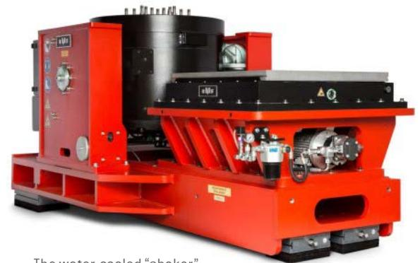
The water-cooled "shaker" used in our test lab
